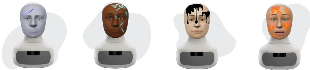
**Figure 1: Exemplified designs on how to leverage robot faces as affective visualisation design to convey environmental data by incorporating agency: (left) Robot face as graphical user interface, (middle) metaphorical representation of environmental data via loss of leaves as a symbol of death or dripping oil [19] combined with an aging face, (right) blazing fire combined with negative facial expressions.**
